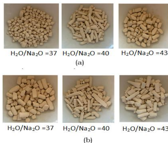
Gambar 2. Zeolit Hasil Pengembangan (a) T_{\text{kalsinasi}} = 570^{\circ}\text{C} dan (b) T_{\text{kalsinasi}} = 670^{\circ}\text{C}
